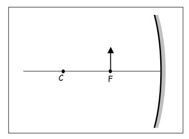
When object is at F, the reflected rays are \_\_\_\_\_ to each other.
